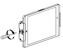
It is not recommened to tighten security screw more than 0.5N m to elimnate risk of hardware damage
