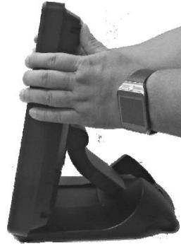
5. Press the circled section with two thumbs and pull by force the two sides of the locking hook with two forefingers as indicated by the arrow.
