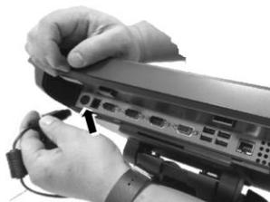
12. Cover the bottom I/O interface and gather the I/O cables to the circled cable arrangement area, as shown below.
