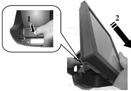
4. When the display goes down to a degree, loose the base-folding lever, as shown in the direction as indicated by the arrow below.
