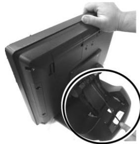
15. Shield the I/O cable arrangement area on the neck of the base stand with the neck cover.
