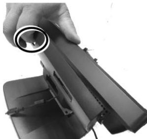
11. Connect the connector of the power adapter to the 12VDC-IN power jack.
