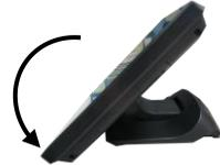
5.3 To tilt screen up or down to your desired angle, please be advised to keep the base steady with one hand to do so. Do NOT press on the LCD panel while setting up the tilt angle.
